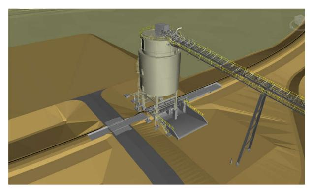
Conceptual Illustration 5: TLO Bin, Loadout Conveyor, TLO Sump and Rail
